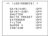
•If both GAIN (0 dB) and GAIN (-3 dB) have been set to ON at the same time, !LED will light on condition that settings other than 0 dB and −3 dB have been respectively selected for the two GAIN items.
